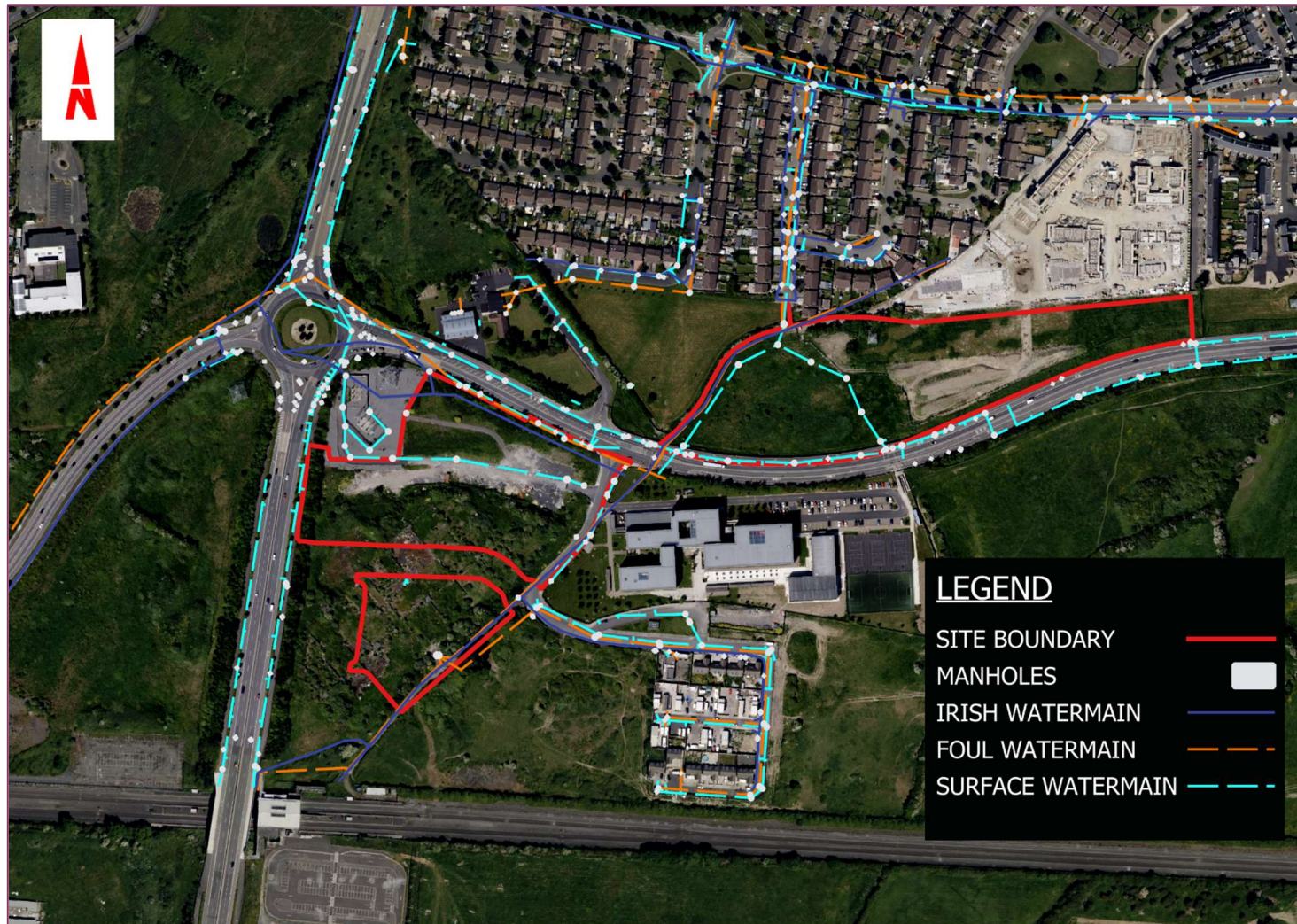
Figure 3-3 Existing Drainage Systems in vicinity of the proposed development sites (source: Uisce Eireann mapping database)
